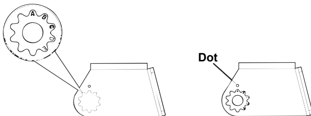
Align plastic ratchets in bracket.
